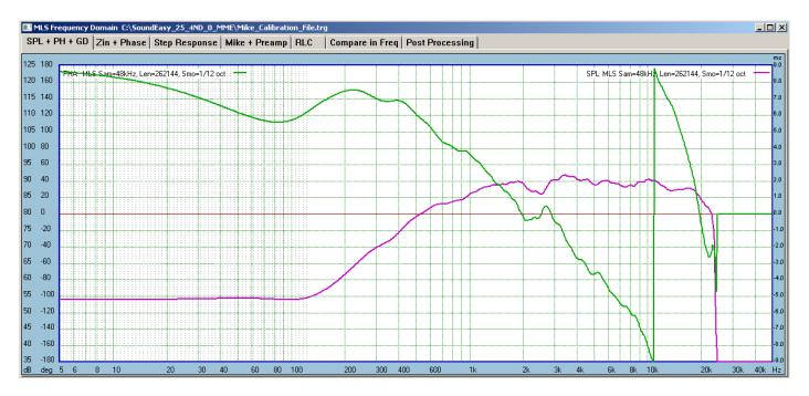
Having done that, the measured phase response becomes the PHASE TEMPLATE for correcting HBT settings. We can now go to HBT screen and correct HBT settings to reflect correctly measured Minimum-Phase phase response.
