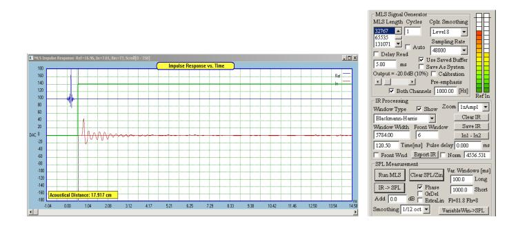
Now, we are grappling with the same question as for the tweeter -how to determine the correct **FFT window placement**? Shown below are three examples of FFT window placement, and corresponding phase response (green curves).
