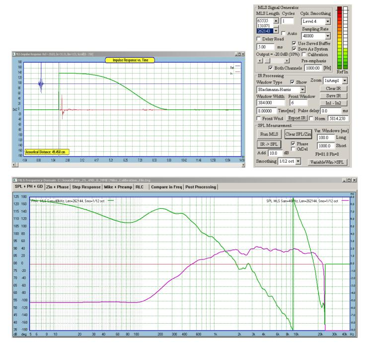
Now, we are grappling with the same question – how to determine the correct FFT window placement?. Shown below are three examples of FFT window placement, and corresponding phase response (green curves).
