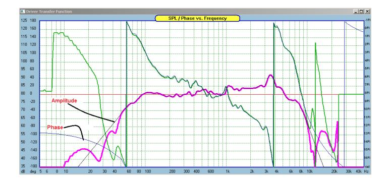
As mentioned before, the IHBT is not sensitive to the attached slopes. We can see this on the three examples shown below. Despite having low-frequency phase slopes (actually SPL slopes translated to phase slope) attached at different frequency points and with different slopes, the algorithm always selects Bin 77 with the minimum error.
