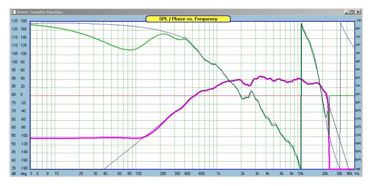
The thin blue curve is the minimum-phase phase response. Please note, that the phase response is clean and extends across the whole frequency range.
