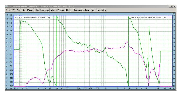
Having done that, the measured phase response becomes the PHASE TEMPLATE for correcting HBT settings. We can now go back to HBT screen and correct HBT settings to reflect correctly measured Minimum-Phase phase response.
