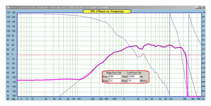
As explained before, in Stage I, the FFT window is placed at 10 arbitrary, but consecutive time samples, and resulting phase responses are supplied to the IHBT algorithm. This way, we obtain 10 SPL responses and one of them will be the best match with the originally measured SPL.
