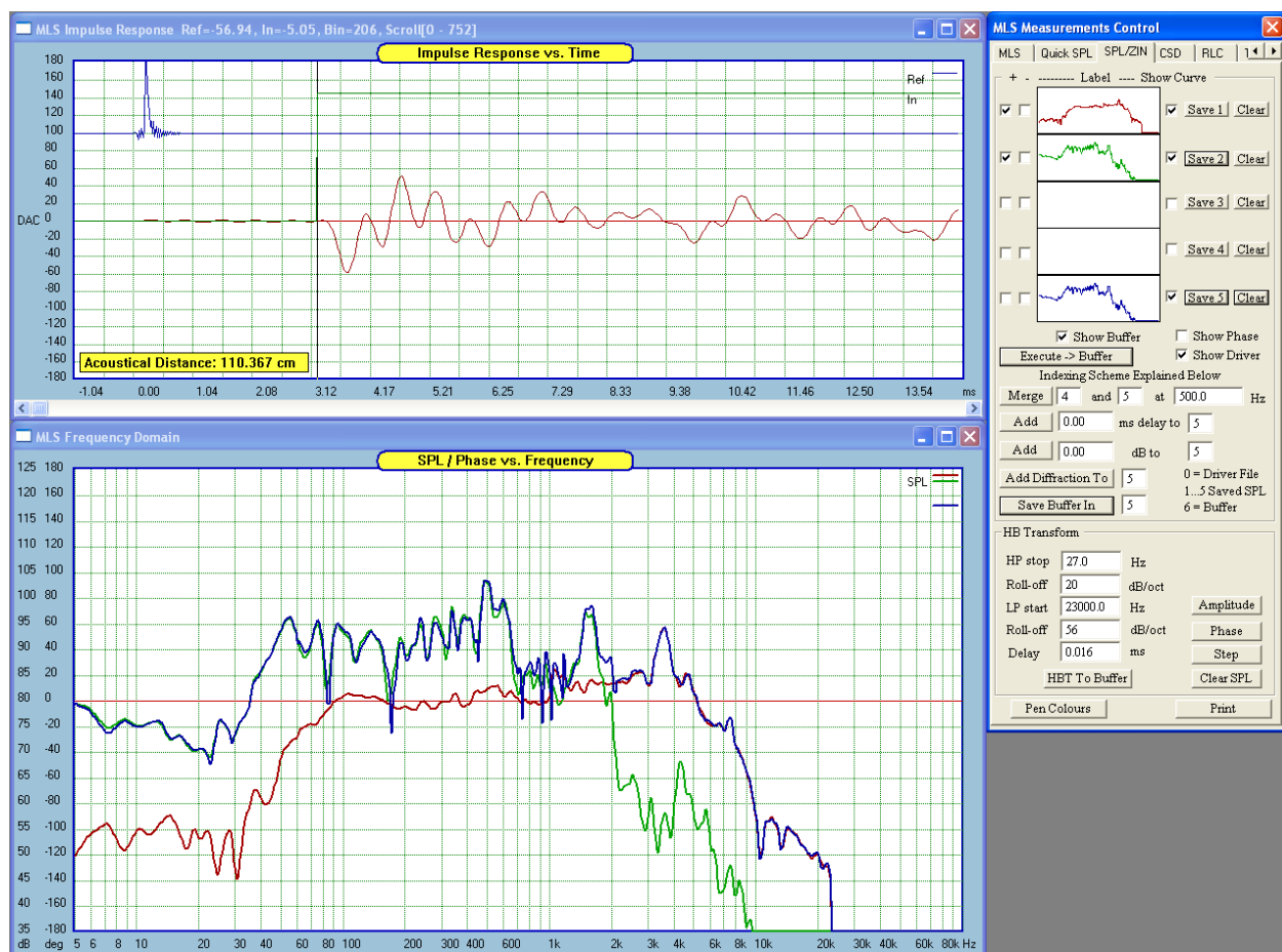
Figure 16.12. SPL (bottom plot) from Fig 10 + 11 added together (blue plot).
