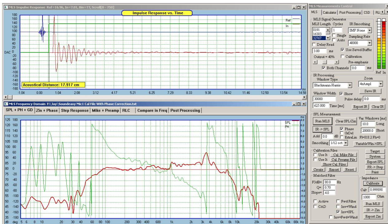
Figure 16.2 Example of SPL/phase response (1/12 oct smoothing) with echoes due to window of 30000 samples.
