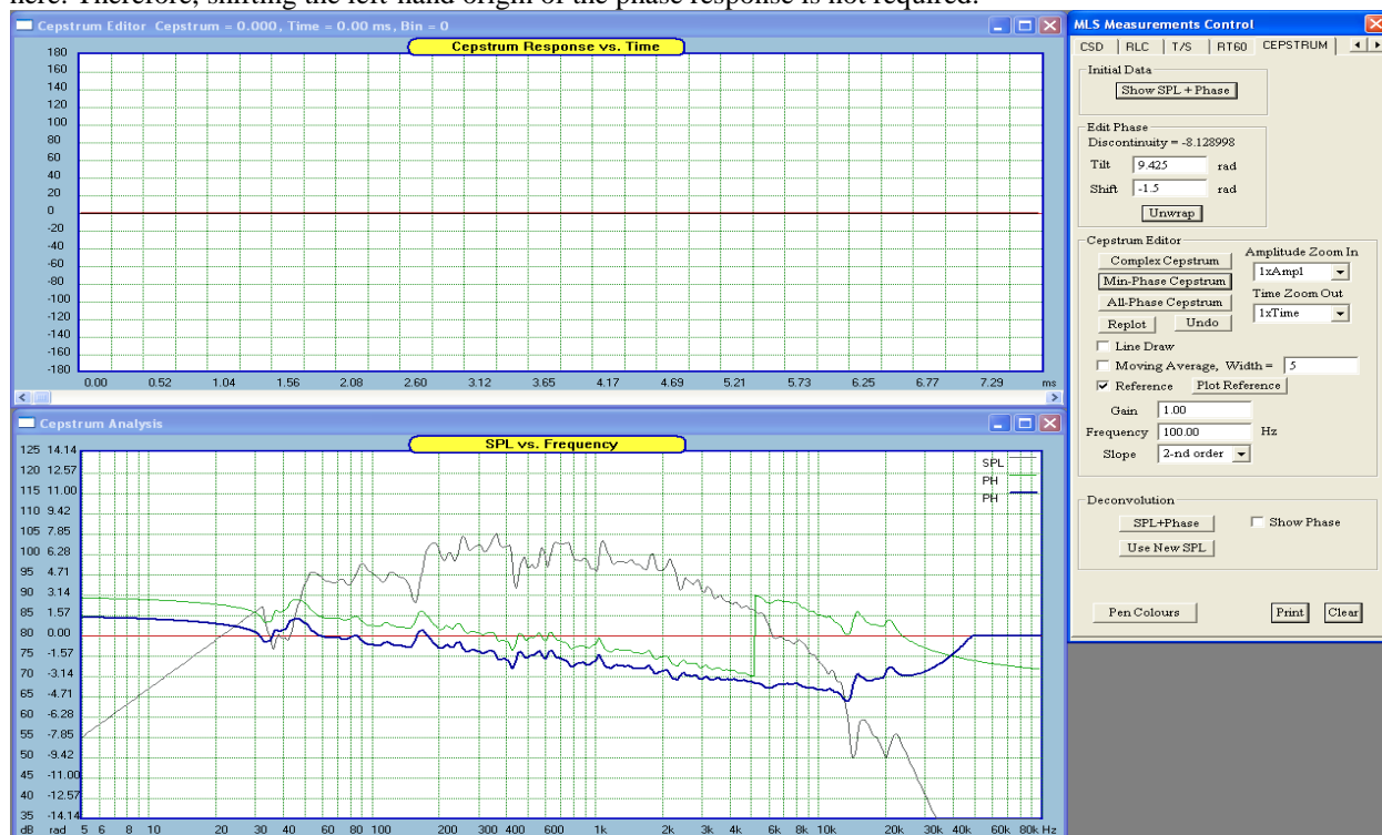
Figure 16.123 “Unwrapped” and adjusted (shift = -1.5) phase response.
