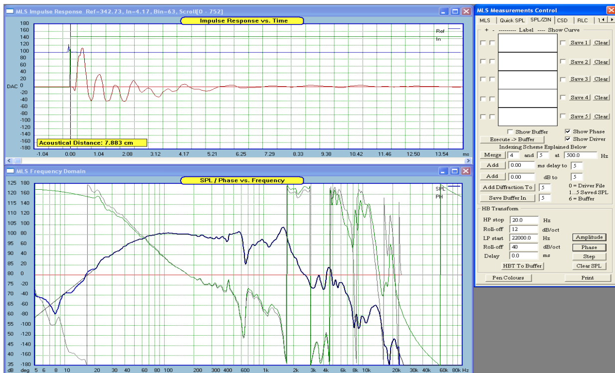
Figure 16.132. Close-mike measurements of a wooferdriver.
