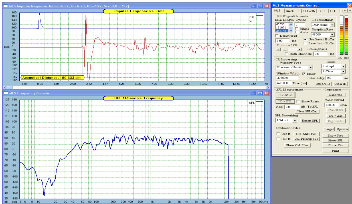
Figure 16.139. Loudspeaker shown above is a wide-band system exposed to a number of room reflections. In fact, this is the same driver, that was used to calculate RT60 – “Figure 16.62. RT60 calculated without noise reduction techniques”. So the echoes are numerous.
