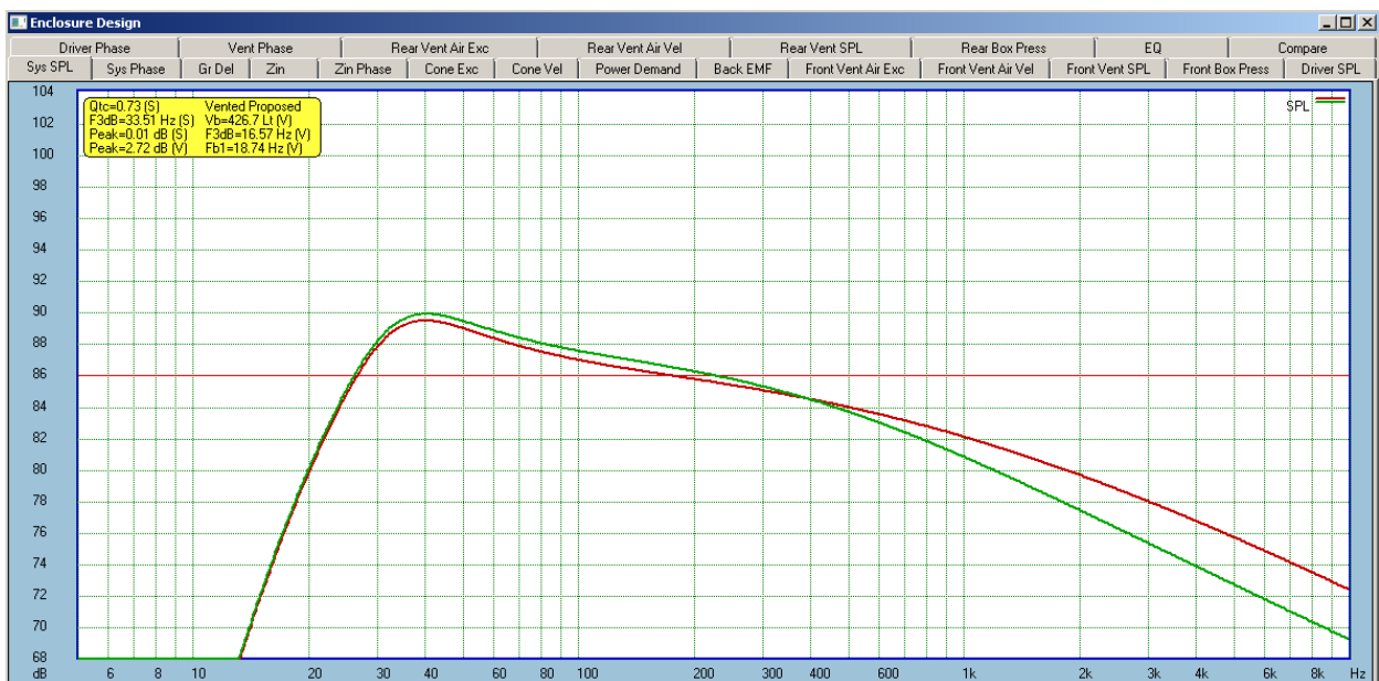
Figure 16.223. Green – Motor Impedance Model, Brown – Semi-Inductance Model.
