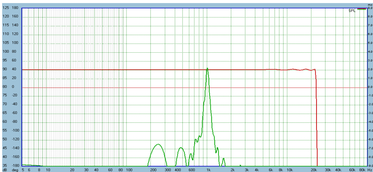
Figure 16.186. Green – sine wave response after FFT, Brown – MLS response after FFT.
