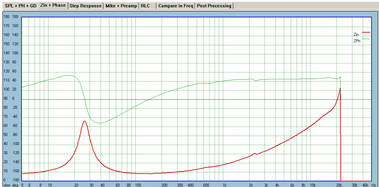
Figure 16.218. Input impedance curve measured with R=540\Omega .
