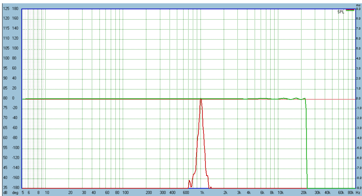
Figure 16.189. Brown – sine wave response after FFT, Green – MLS response after FFT. Note, almost the same level of 80dB.
