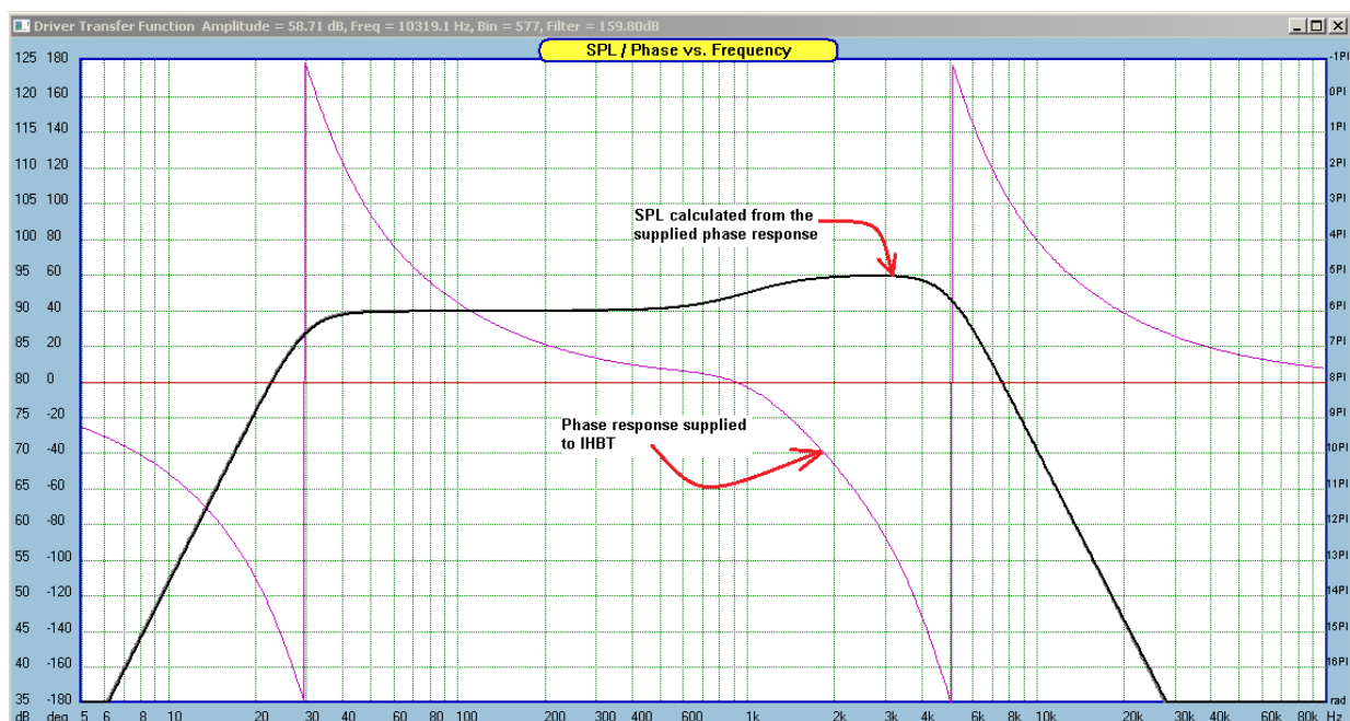
Figure 16.229 SPL extracted from phase response of a simple filter 1.
