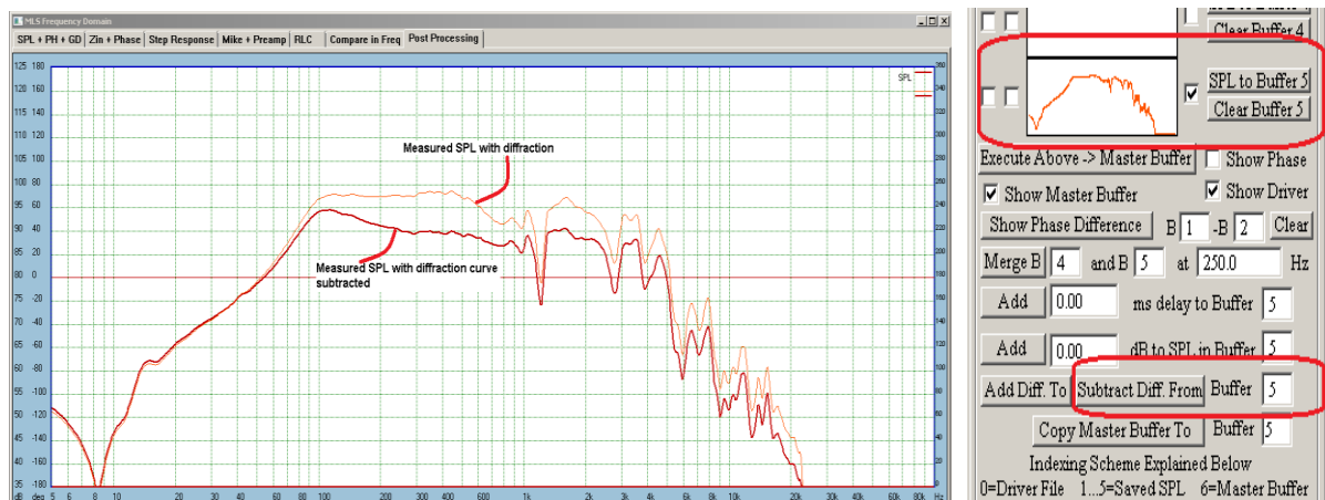
Figure 16.247 Example of subtracting diffraction from SPL in Buffer 5.
