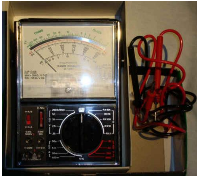
Figure 16.202. Multimeter used to measure 2.83Vrms for 1W/1m at 8ohm measurements
