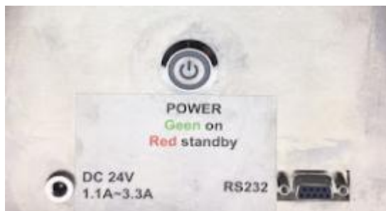
Figure 16.289. ANSI Turntable components – front panel and power supply.
