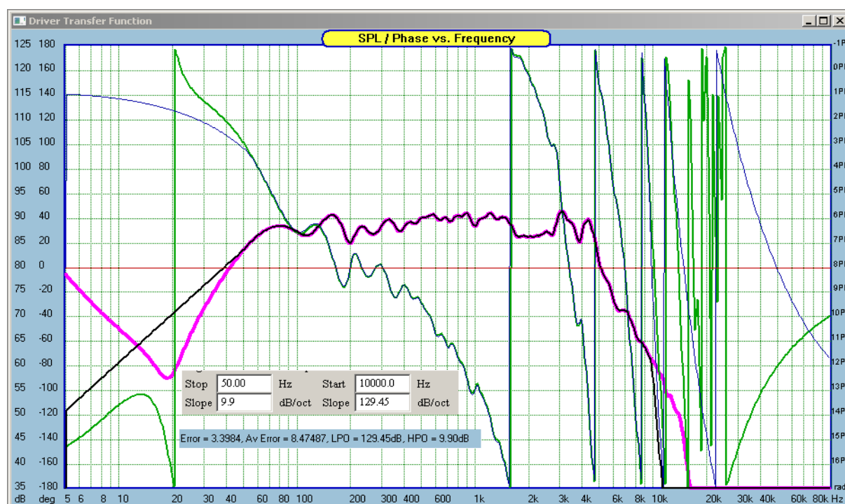
Figure 16.324. Example of visually very good phase match at 10kHz attachment point.
