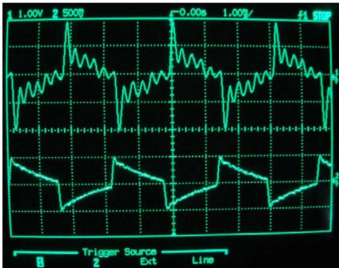
Figure 19.16. Square wave passed through amplitude-linearizing system.
