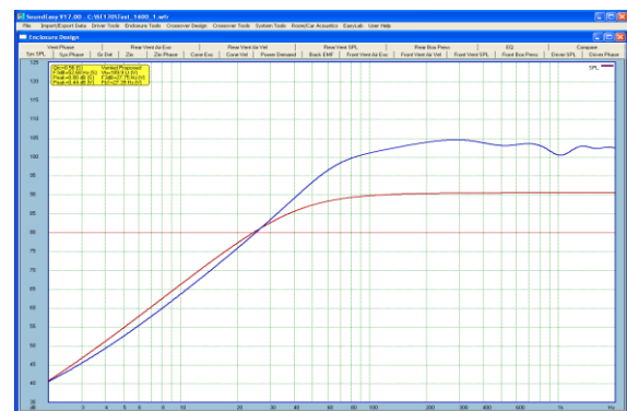
Four drivers connected in-series and in-parallel
