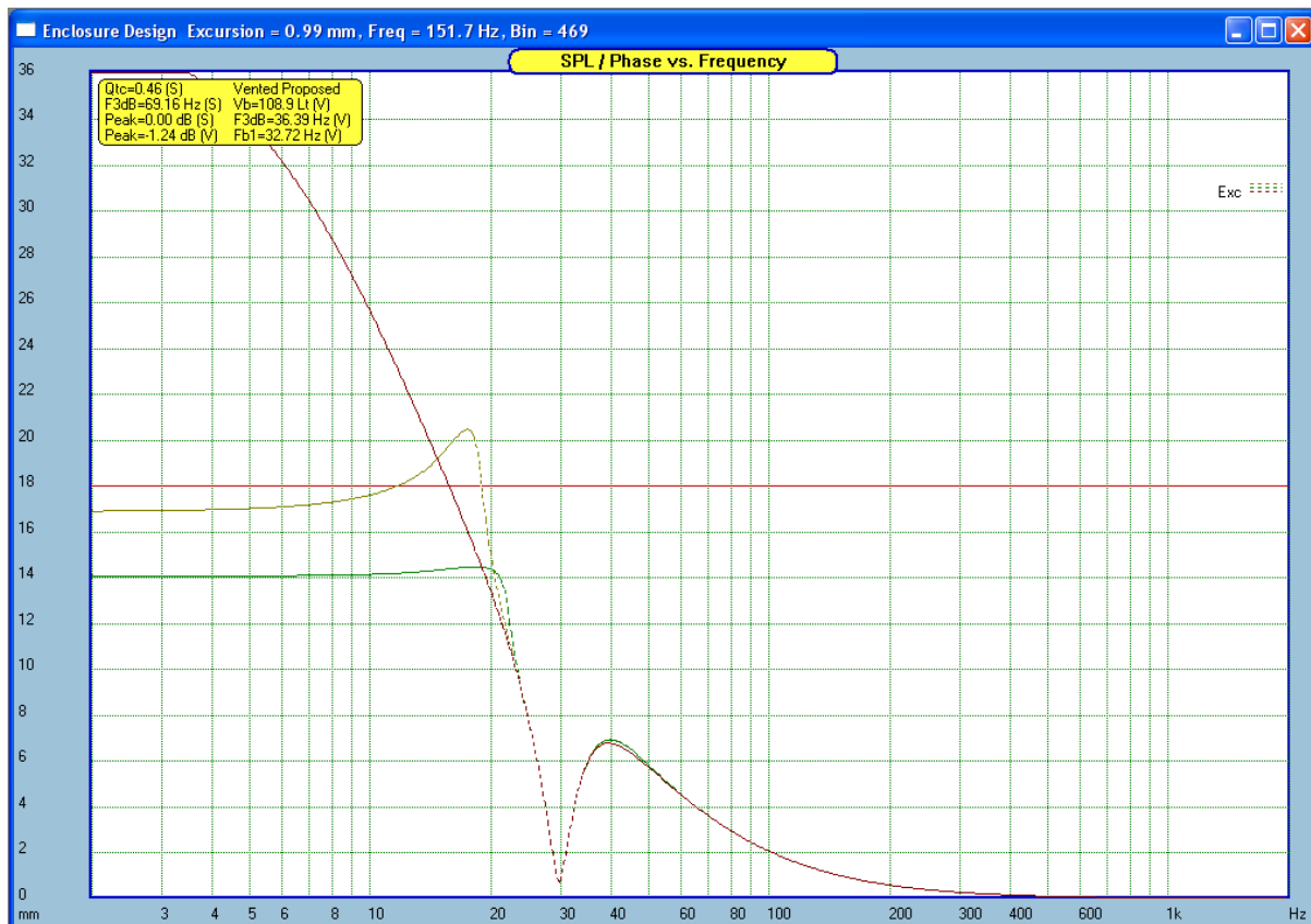
Figure 4.63. Cone excursions. “light brown”- Cas(x) nearly linear, “green” – Cas(x) soft clipping, “red” – BL(x) and Cas(x) completely linear..
