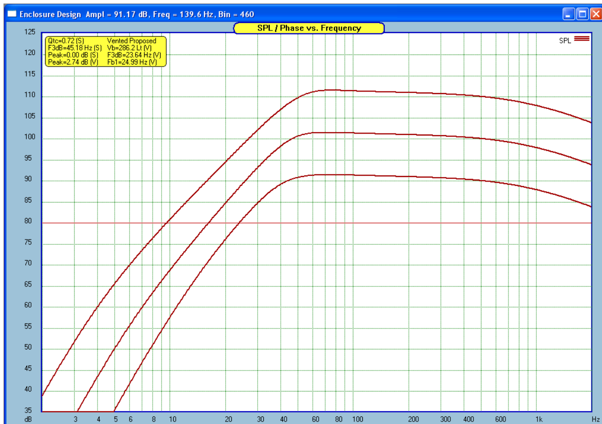
Figure 4.52. SPL for port diameter of 3cm, @1W, 10W and 100W input power
