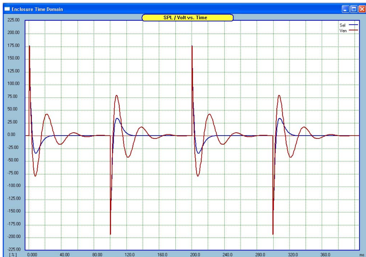
Figure 6.3 Transient response of sealed and vented boxes at 5Hz
