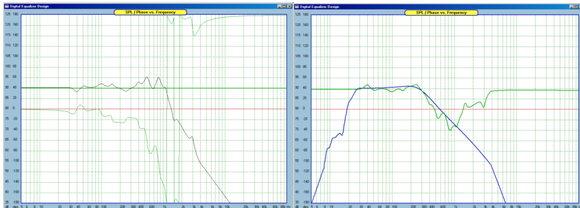
Fig 9.33. Modified driver (left) does not create tails (right)
