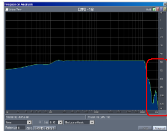
Fig. 19 – measured frequency response of the artificial mouth system after equalization
