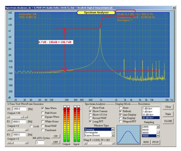
It looks asymmetrical, and on the low-side the SNR is estimated to be 136dB. On the high-side, it seems to be around 155dB.
