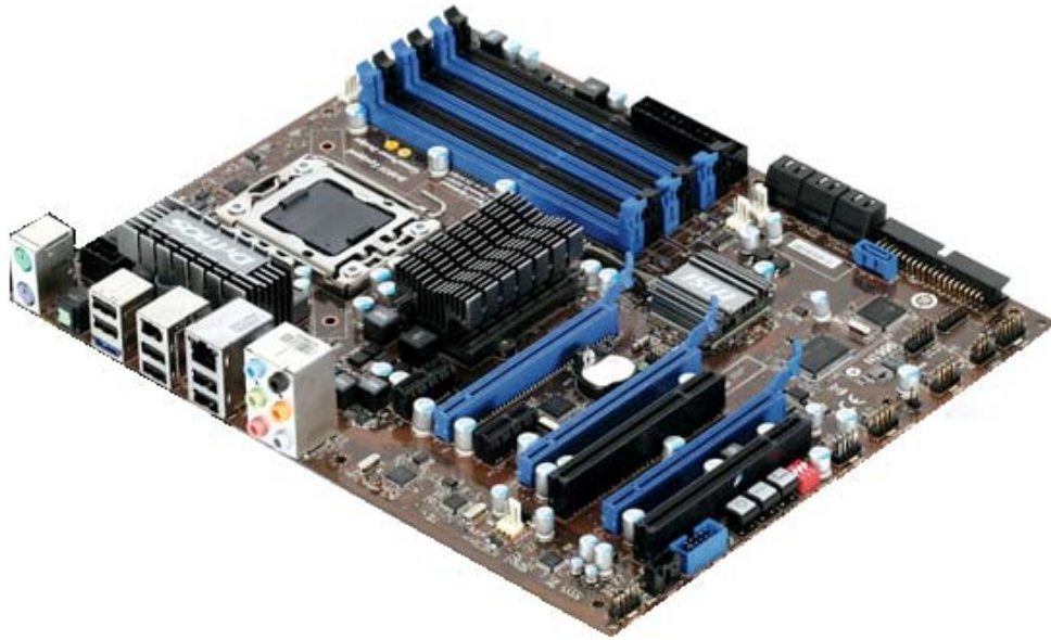
Figure 3. Motherboard MSI X58 Pro-E Series with 2 x PCI slots. http://au.msi.com/product/mb/X58-Pro-E.html
