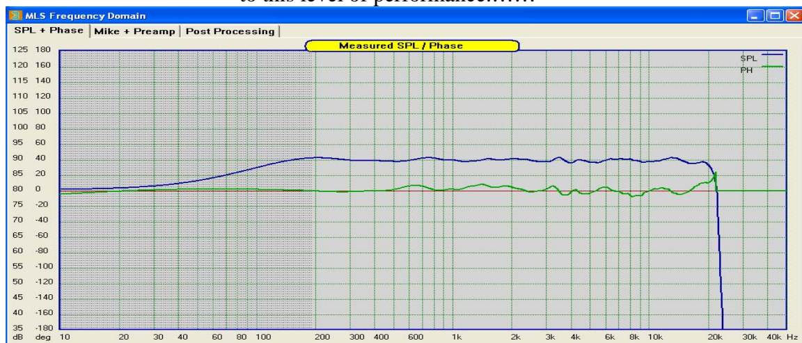
Figure 30. Equalized SPL and phase in 2-way system.
