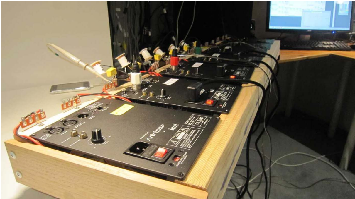
7 PWR-ICE amplifiers are mounted on a frame for easy access.
