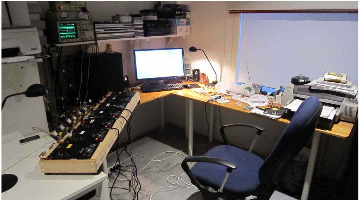
Signal Generator, CRO, PC with Ultimate Equalizer.
