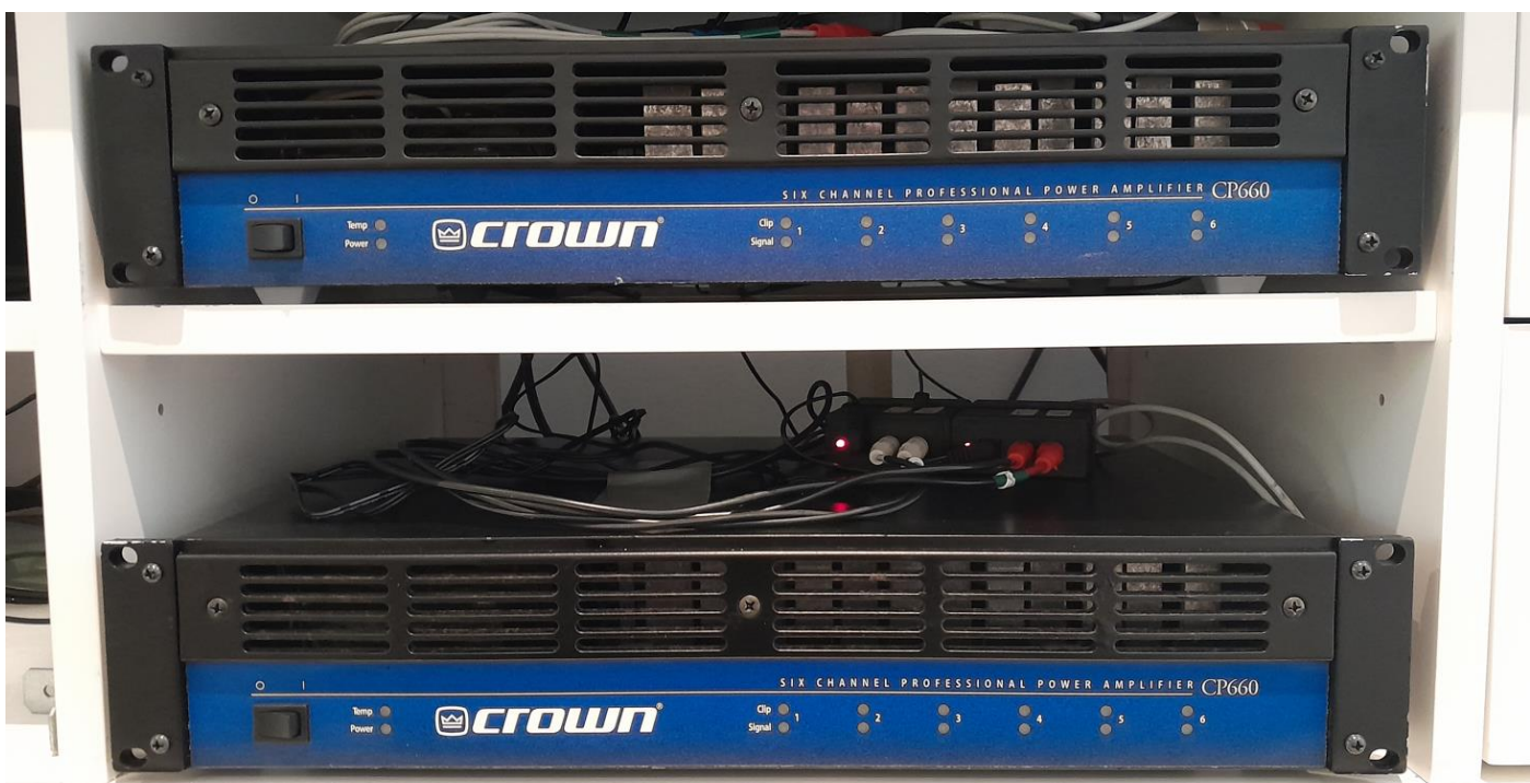
CP660 amplifiers installed in the HT cabinet.
