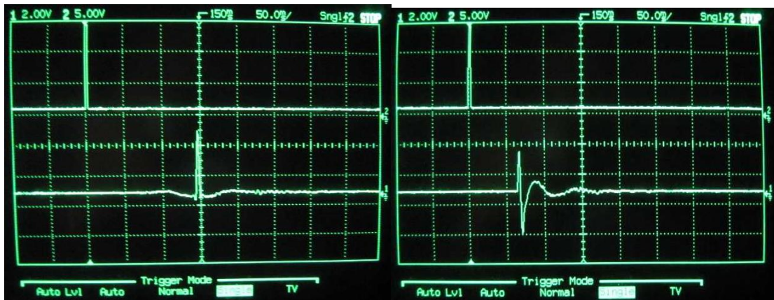
5ms Impulse in Linear-Phase Mode and Minimum-Phase Mode
