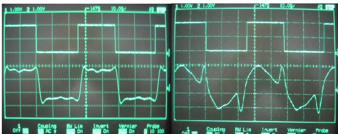
20Hz square wave: Linear-Phase Mode and Minimum-Phase Mode
