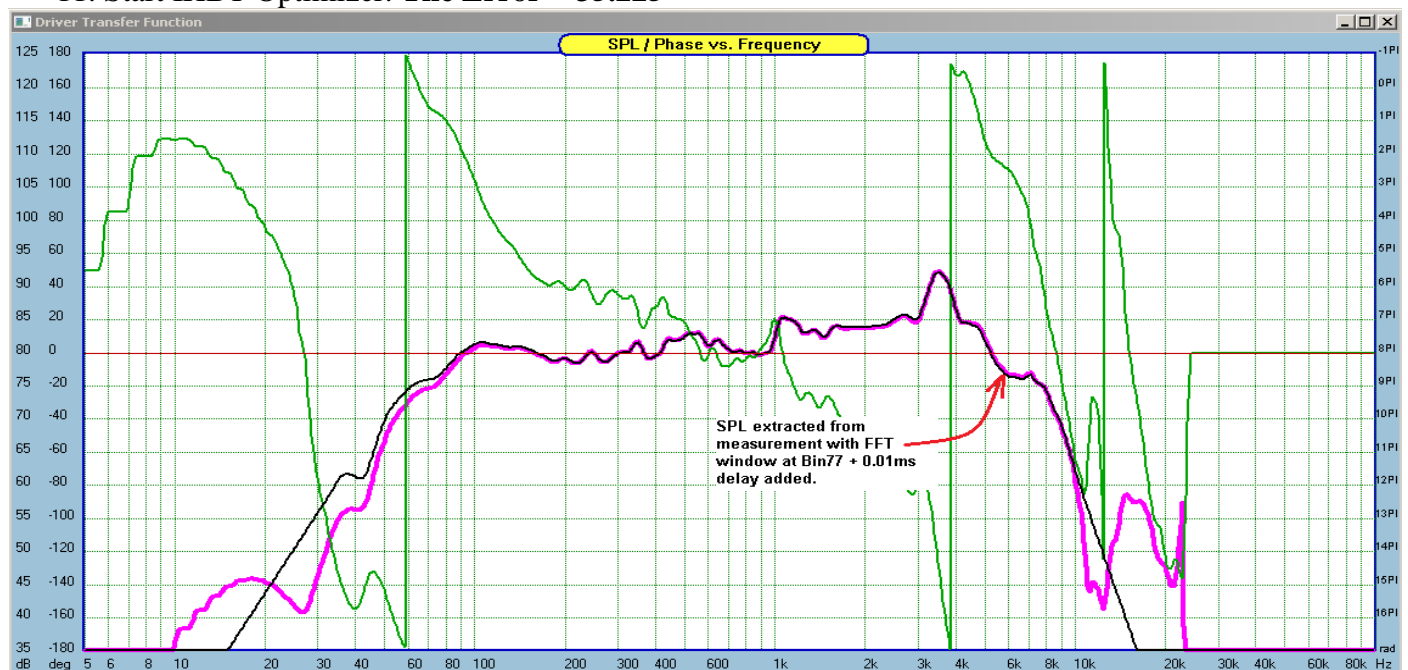
Fig 9. SPL extracted from measured phase with FFT window at Bin77+ 0.01ms delay.
