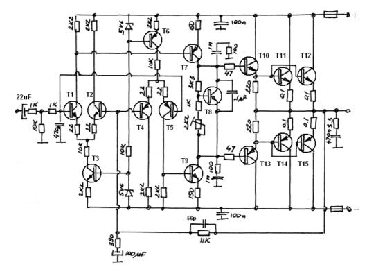
There are 2 modules of 200W amplifiers in the system. The output power is easily controlled by supply rail voltage. The 2.2kohm variable resistor is used to adjust idle current of the output transistors to 25mA combined.
