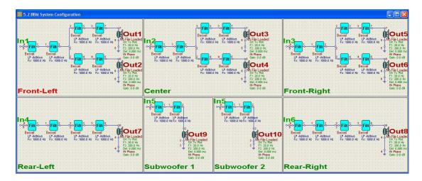
Picture above, shows corresponding BBM System Configuration screen, with two subwoofers serviced via SPDIF DAC on outputs 9 and 10.
