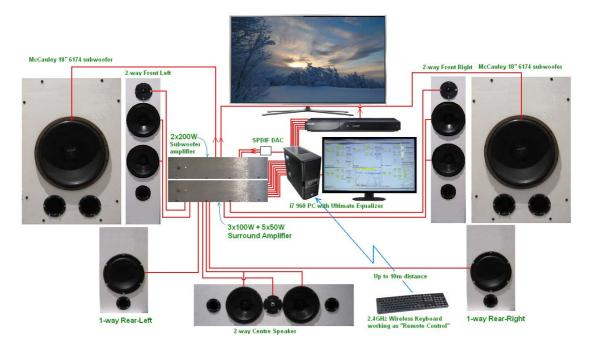
The SPDIF DAC is shown as separate component, but it would be typically built into the amplifier – in this case – subwoofer amplifier.
