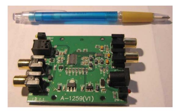
In our 2-way, WTW loudspeakers, the 8 ohm tweeter is powered by a 50W amplifier Kit KC5150 from Jaycar Electronics, Melbourne Australia.
