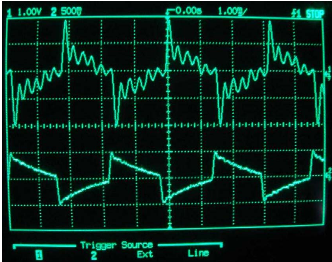
Figure 7. Square wave passed through amplitude-linearizing system. Trace 1 – loudspeaker alone. Trace 2 – SPL-equalized loudspeaker.
