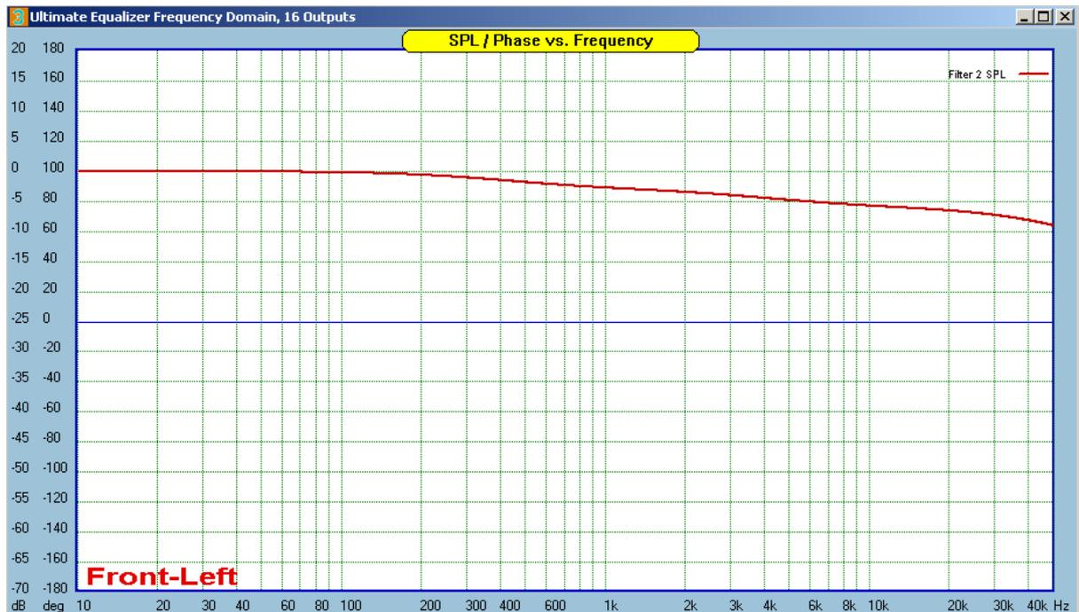
Figure 11. Correction curve based on 3-segment Q-Parametric filters to approximate Moller's correction
