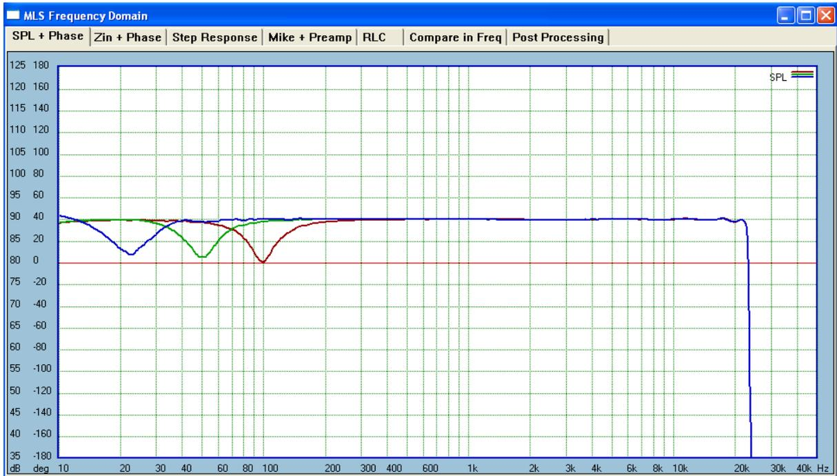
Figure 9. The same -10dB notch at 100/50/20Hz played through 8P version with 512buffer
