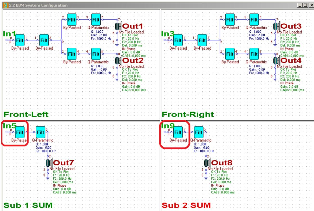
Figure 3. Typical 2-way system set-up as 2.1 with single subwoofer augmentation.
