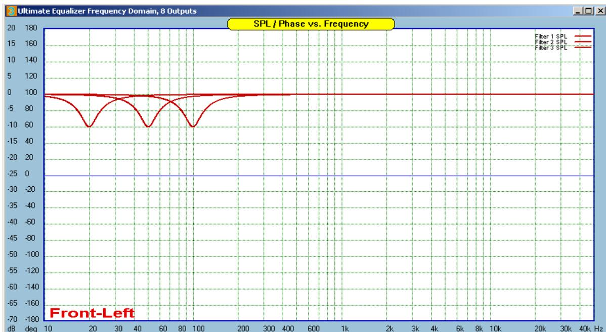
Figure 6. -10dB notch at 100Hz, 50Hz and 20Hz designed in System Design screen
