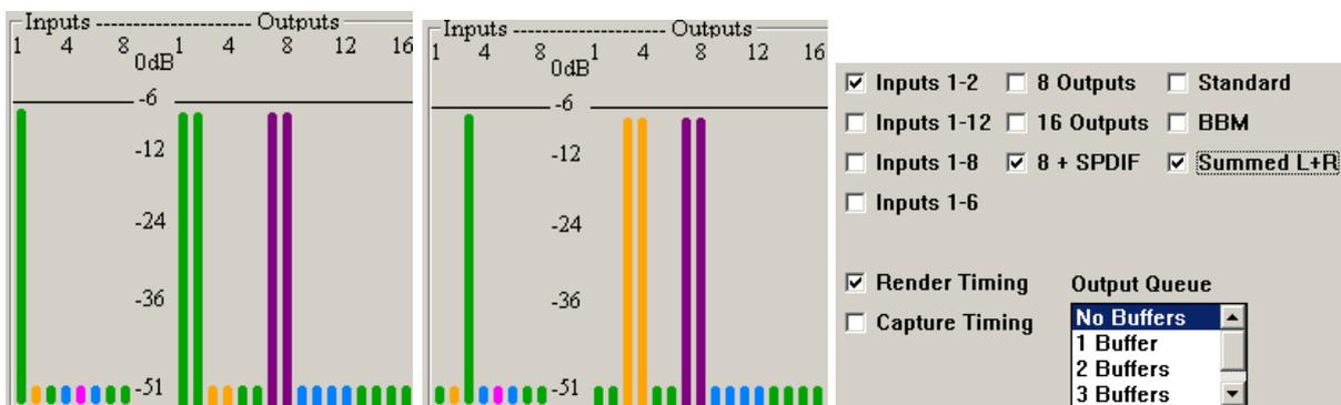
Figure 4. Signal flow when only left/right channel is active, and Preferences settings.
