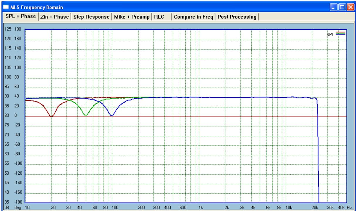
Figure 7. The same -10dB notch at 100Hz, 50Hz and 20Hz played through 16P version with 1024 buffer.
