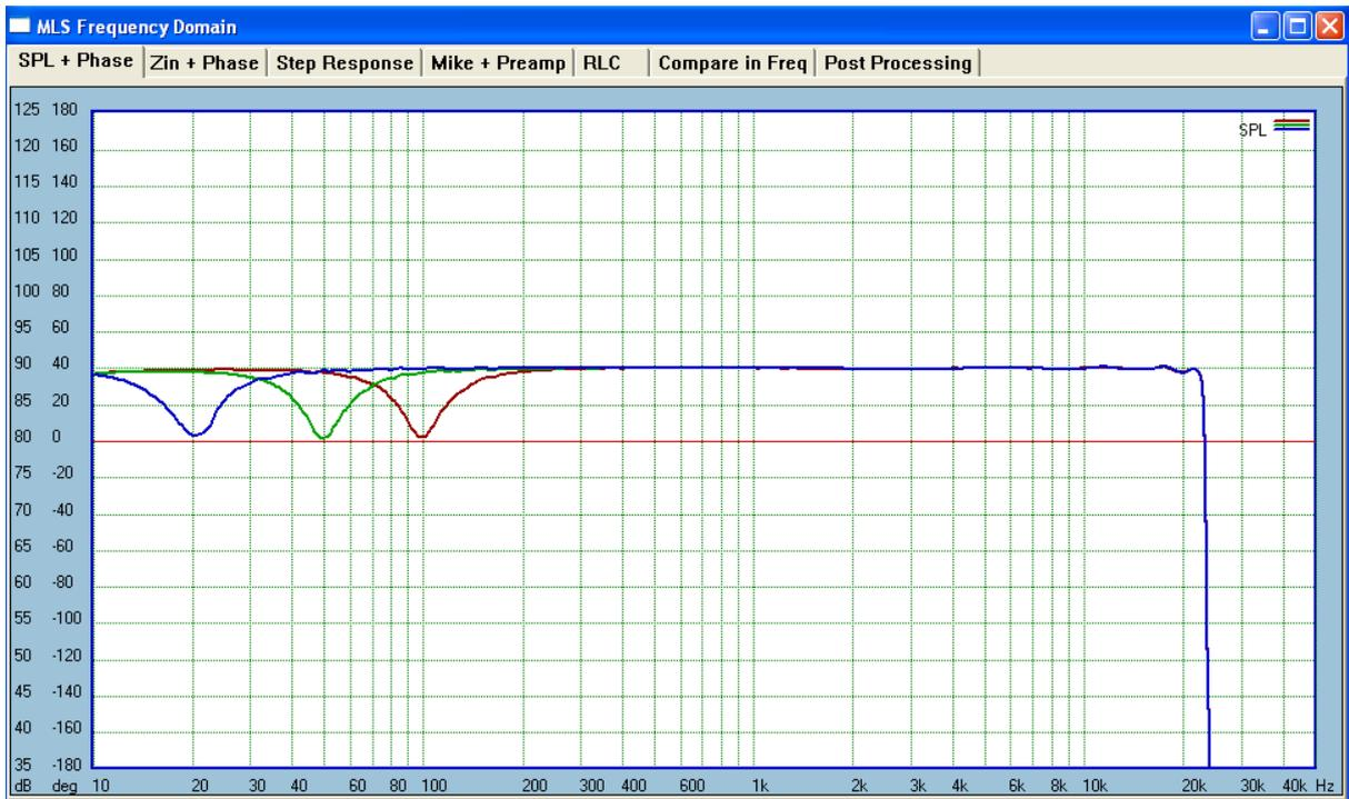
Figure 8. The same -10dB notch at 100Hz, 50Hz and 20Hz played through 16P version with 512 buffer.
