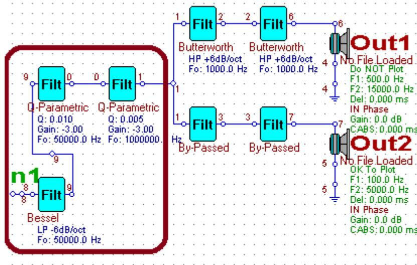
Figure 10. Introduction of 3-segment Q-Parametric filters to approximate Moller's correction
