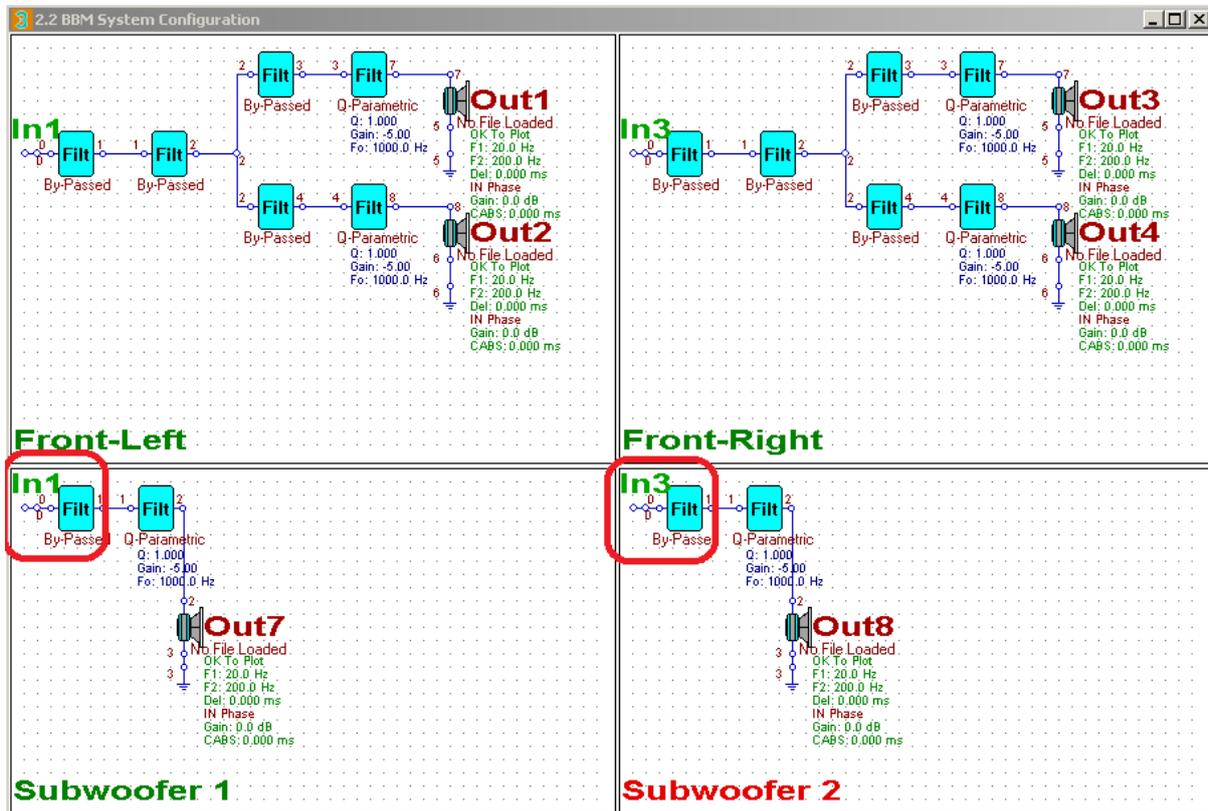
Figure 1. Typical 2-way system set-up as 2.2 with left/right subwoofer augmentation.
