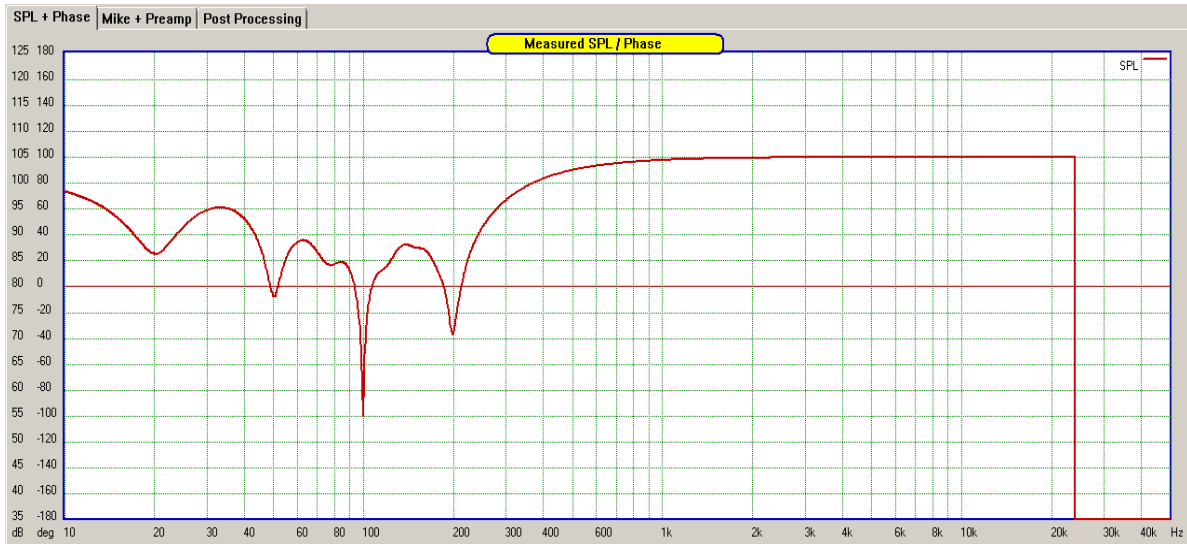
Figure 2. Experimental FIR filter with four notches implemented in low bass resolution FIR.
