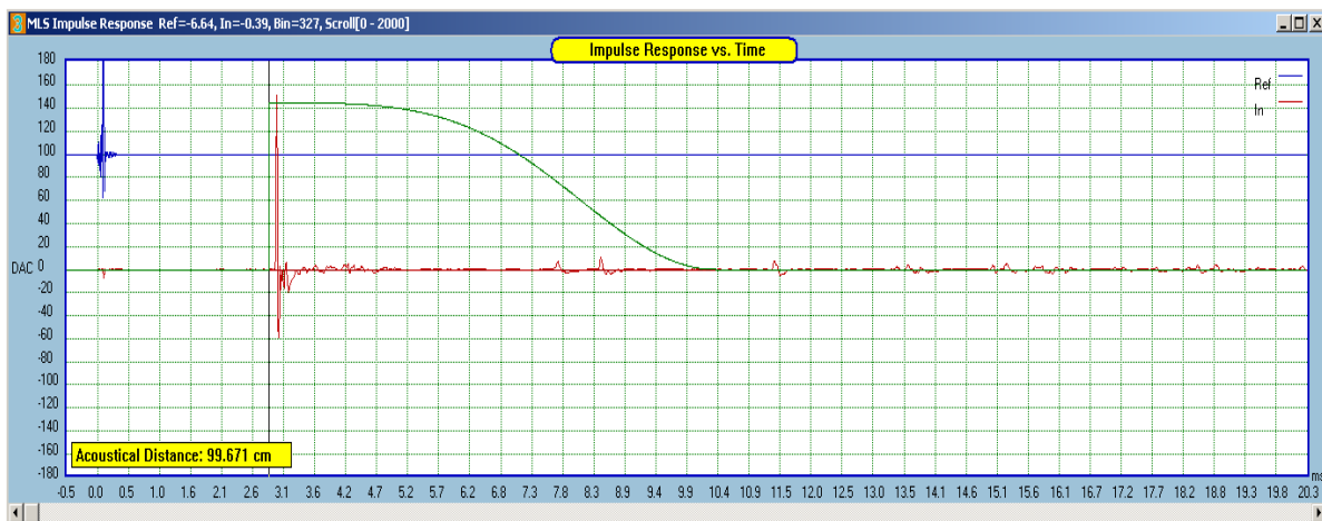
Figure 33. Start of the FFT window (9 bins to the left).
