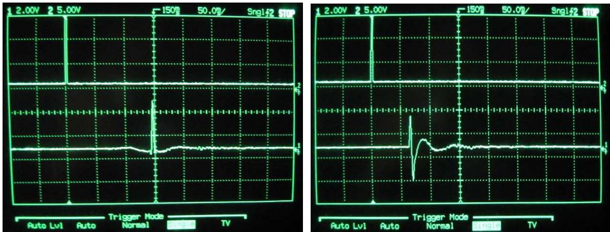
Figure 21. 2ms Impulse in Linear-Phase Mode and Minimum-Phase Mode
